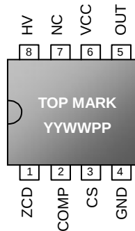
SOP-8 / DIP-8 (TOP VIEW)
